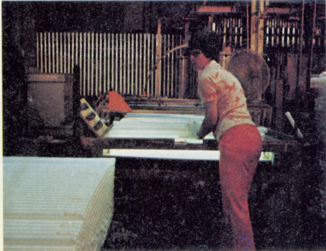
Phosphor coating uniformity is very important to fluorescent tube performance and is closely monitored during the manufacturing process.
