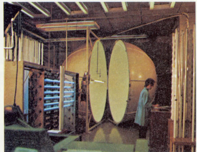
Light output is measured precisely by spherical photometer in GE lab.
