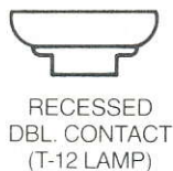
Figure 4. Bases for Fluorescent Lamps.
